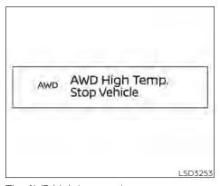
The AWD high temperature message may be displayed while trying to free a stuck vehicle due to increased oil temperature. The driving mode may change to 2-wheel drive. If this message is displayed, stop the vehicle with the engine idling, as soon as it is safe to do so. Then if the message turns off, you can continue driving.
