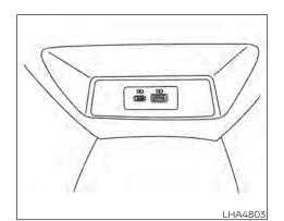
There is a USB/iPod® charging port located on the rear center console. This port will charge compatible devices.
