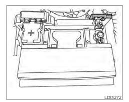
Your vehicle is equipped with a variable voltage control system. This system measures the amount of electrical discharge from the battery and controls voltage generated by the generator.
