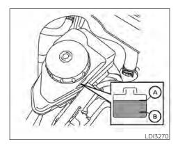
For additional information on brake fluid specification, see "Recommended fluids/ lubricants and capacities" (P. 10-2).
