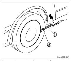
Removing wheel cover (if so equipped)
