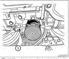
③ Oil filter (2.0L 4 cylinder (KR20DDET engine model))
