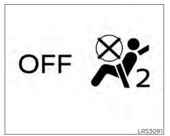
7 If the booster seat is installed in the front passenger seat, place the ignition switch in the ON position. The front passenger air bag status light \*\* \*\* may or may not illuminate, depending on the size of the child and the type of booster seat being used. For additional information, see "Front passenger air bag and status liaht" (P. 1-57).
