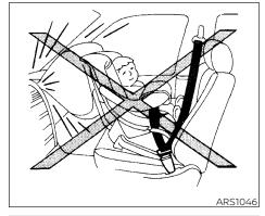
Even with the NISSAN Advanced Air Bag System, never install a rearfacing child restraint in the front seat. An inflating front air bag could seriously injure or kill your child. For additional information, see "Child restraints" (P. 1-23).
