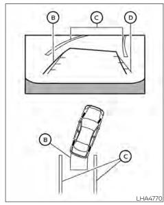
3. Slowly back up the vehicle adjusting the steering wheel so that the predicted course lines (B) enter the parking space (G).
