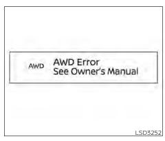
If any malfunction occurs in the AWD system while the engine is running, messages are displayed in the meter.
