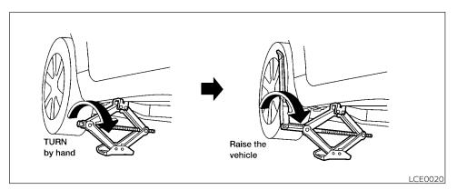
3. To lift the vehicle, securely hold the jack lever and rod with both hands. Carefully raise the vehicle until the tire clears the ground. Remove the wheel nuts, and then remove the tire.
